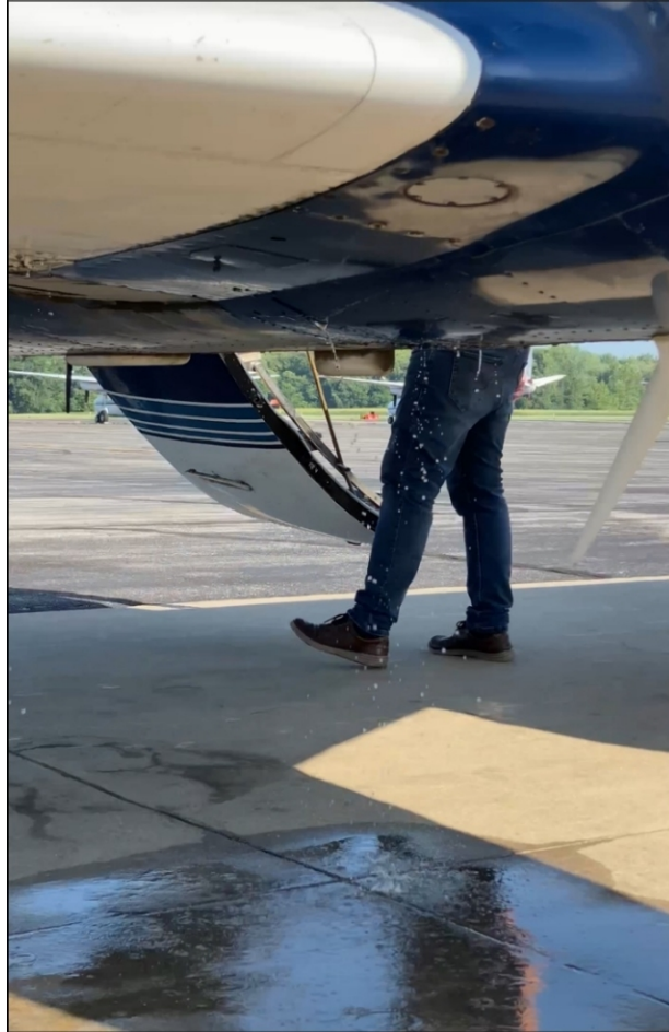
Figure 1: Video screen capture of the fuel leak provide by the lineman witness.
